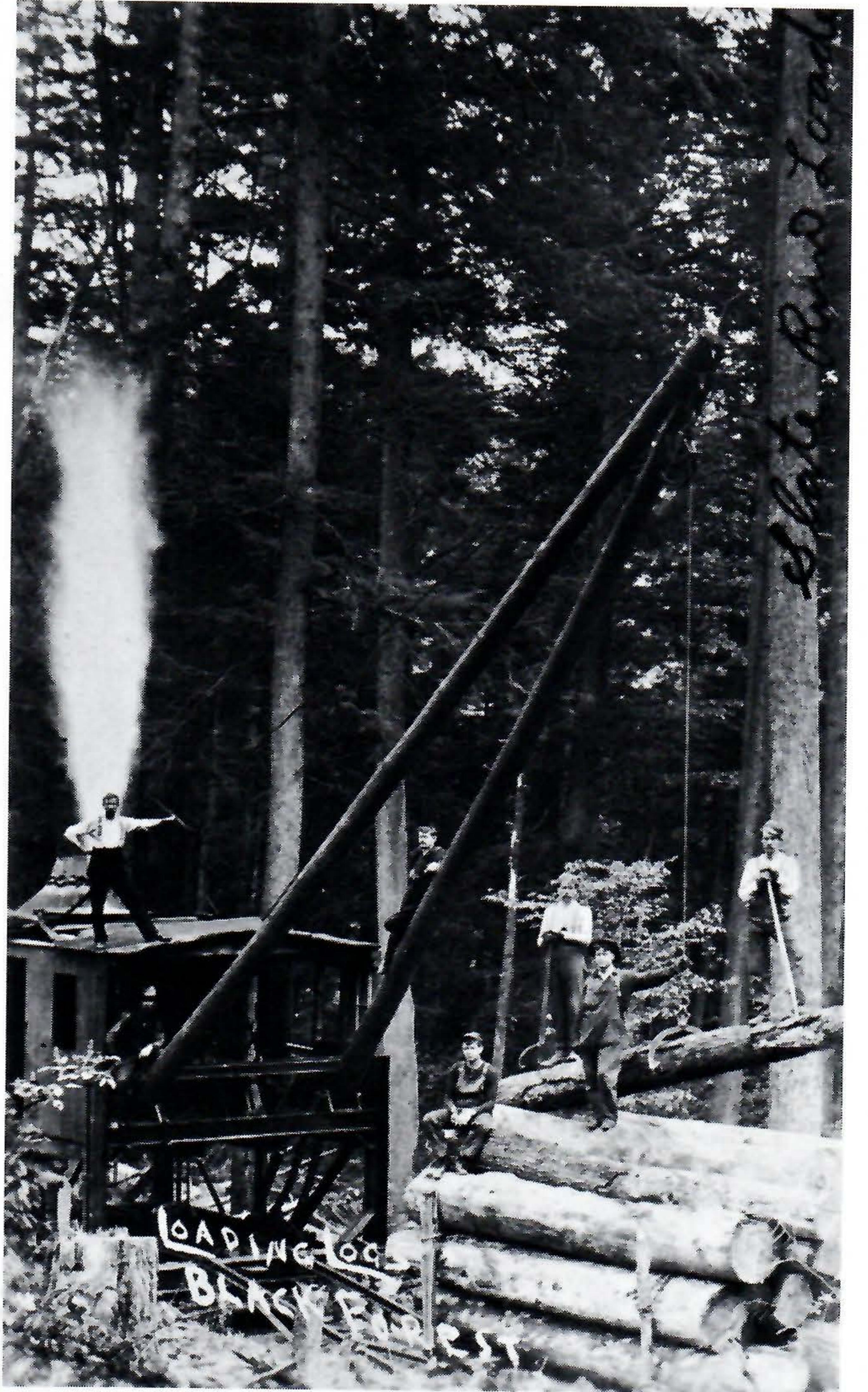
The Slate Run Railroad used a McGiffert log loader. By using the loader and side stakes, the narrow gauge freight cars held as much or more than standard gauge cars without stakes. The use of stakes was not common in Pennsylvania. Neither was the use of a McGiffert log loader. Only one other is known in the state, and this may be the same one, second owner. Watson Lands and Lumber Company at Mayburg, Forest County used one in the nineties.
