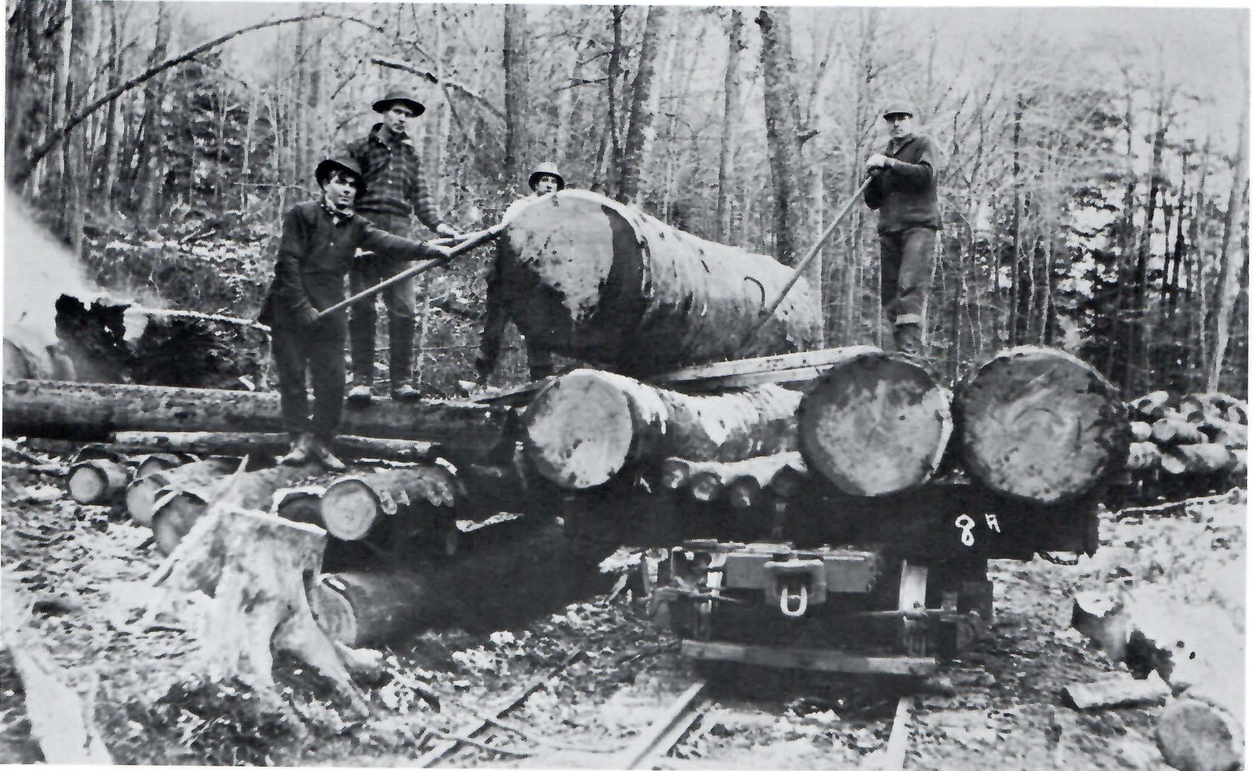
Nelson Caulkins Loading logs without a loader. This is an exceptionally good picture of the method of hand loading logs. After rolling logs like these all day up onto cars, the wood hick was ready for dinner and bed.
