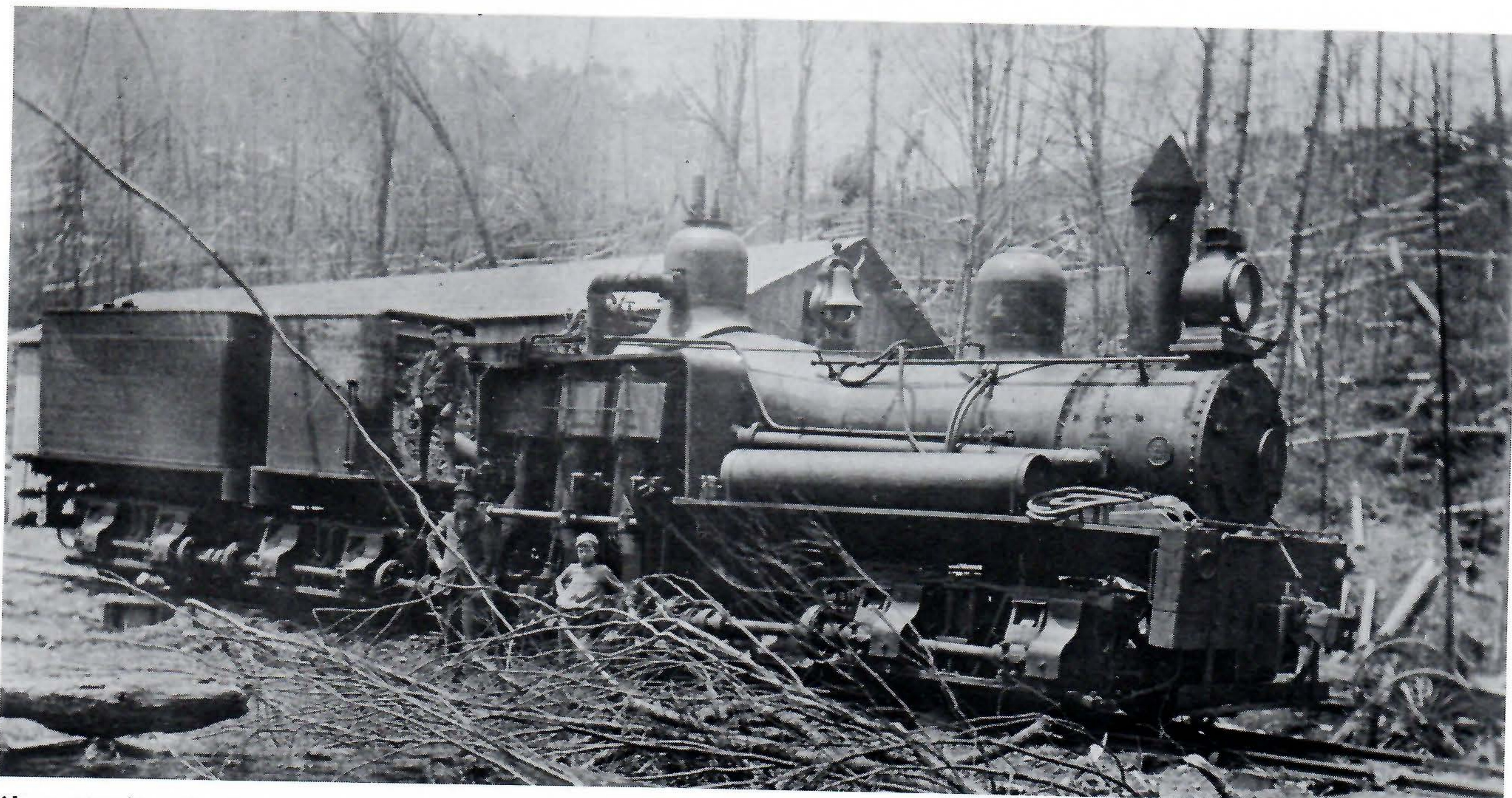
About 1907/8 a fire burned the slashings along Painter Run. Engine No. 4 took a crew of mill hands to help get it under control. The locomotive became trapped and lost its wood cab. A steel cab replaced it. The locomotive was later renumbered No. 202. Harry Lloyd is the boy at the center of the photograph. A few years later a similar fire threatened Leetonia. Thanks to the pasture land around town and stationing men with water buckets on roof tops, flying embers were unable to do any damage.
