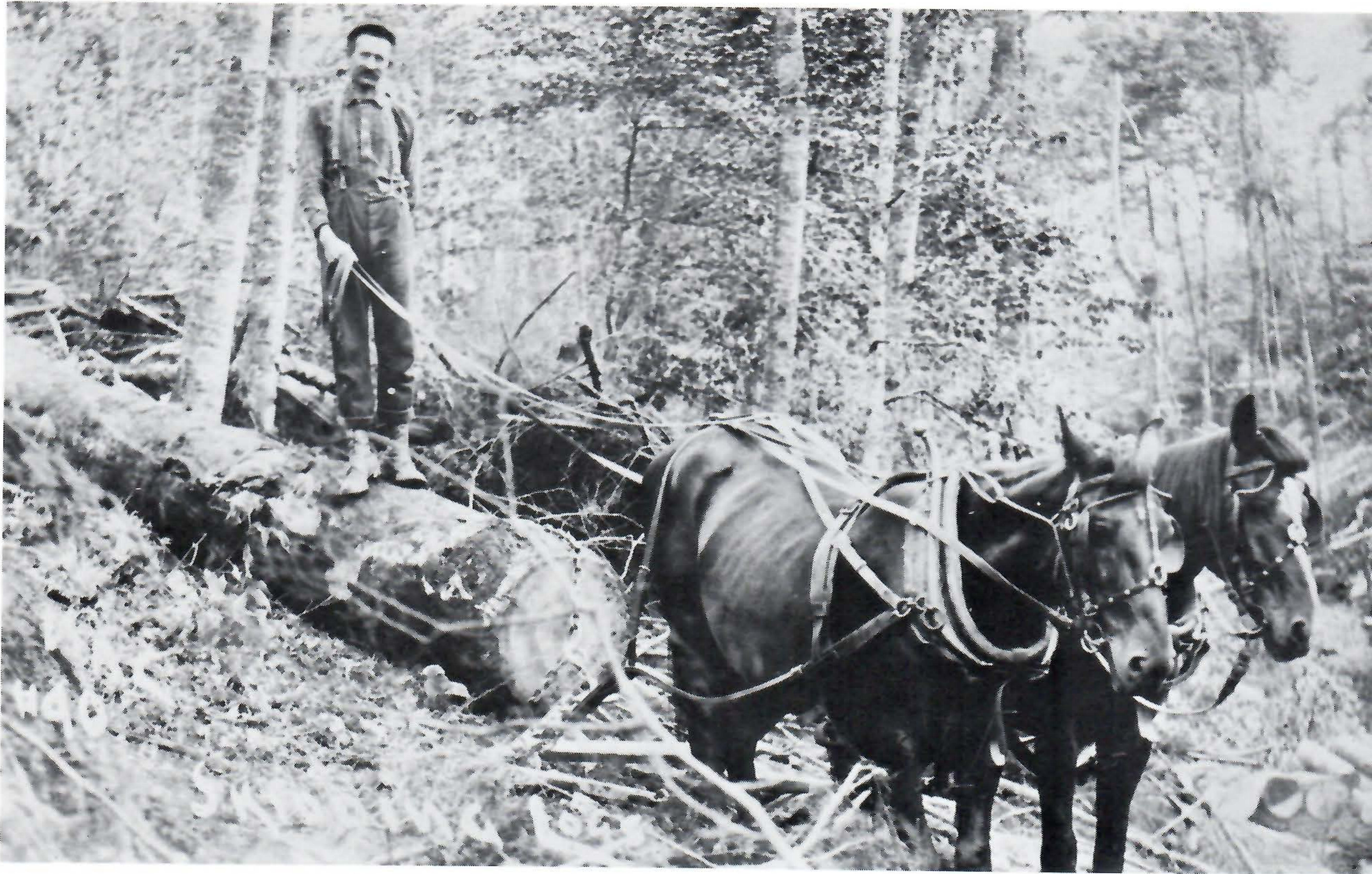
A teamster skids a log to trackside. In 1972 horses are still used to skid scattered logs that can not be readily reached with a tra
