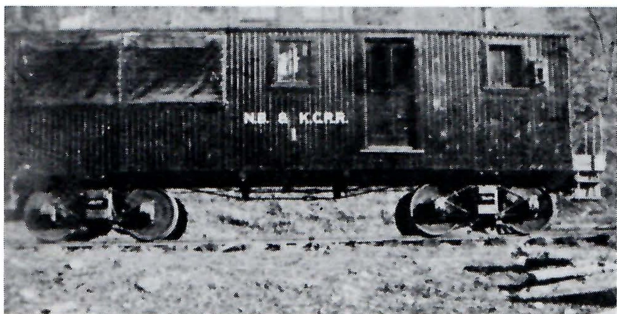
The cupola of the caboose is barely visible in this picture. Canvas covers the open sides of the car. In fair weather the curtains were removed, and there were benches for crew members and wood hicks to sit.
